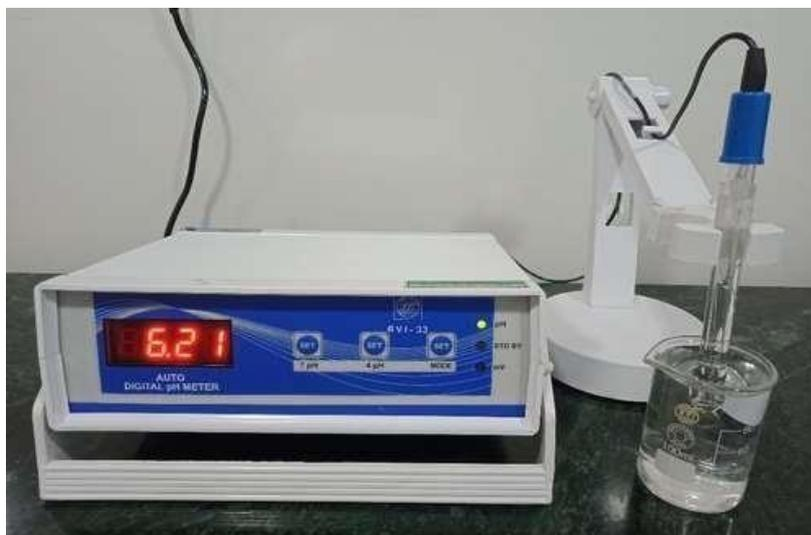
**Figure 1: The pH meter with glass membrane electrode.**
