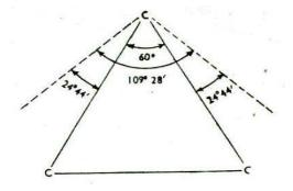
In cyclopropane, the three carbon atoms occupy the corners of an **Equilateral Triangle**. Thus cyclopropane has C—C— C bond angles of  $60^{\circ}$ . This implies that the normal tetrahedral angle of  $109.5^{\circ}$  between any two bonds is compressed to  $60^{\circ}$ , and that each of the
