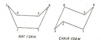
Actually, only one form of cyclohexane is known and not two forms as shown above. The failure to isolate the two forms is **due to rapid interconversions** between them. Such non-planar strain less rings in which the ring carbon atoms can have normal tetrahedral angles are also possible for larger ring compounds.
